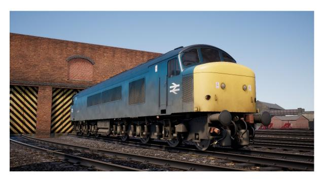
Built by BR's Derby and Crewe Works between 1960 and 1962, the Sulzer Type 4 diesel locomotive were the main passenger locomotives on the Midland Main Line from their introduction until their withdrawal in the early 1980s.
